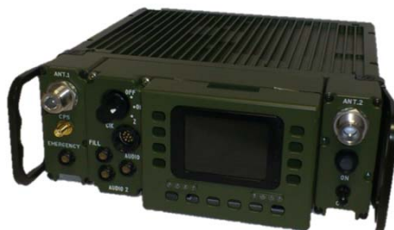
Swave™ Manpack/Vehicular 2 Ch: 30-512 MHz 20W Range Extension with Mission Modules
